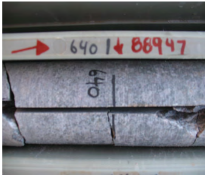
Figure 4. Sample number on core tray at start of the 2.0 m sample interval.
