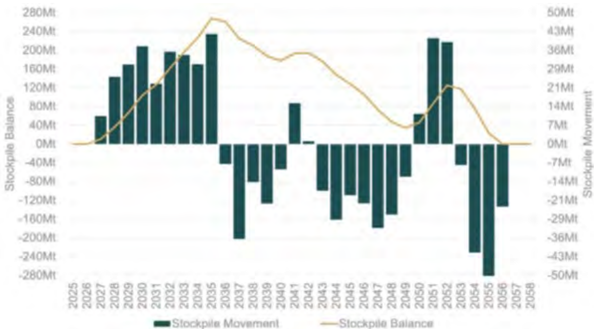
Figure 4-8: Movement of Ore to and from Stockpiles—Probable Ore Reserves and Inferred Mineral Resources model.
